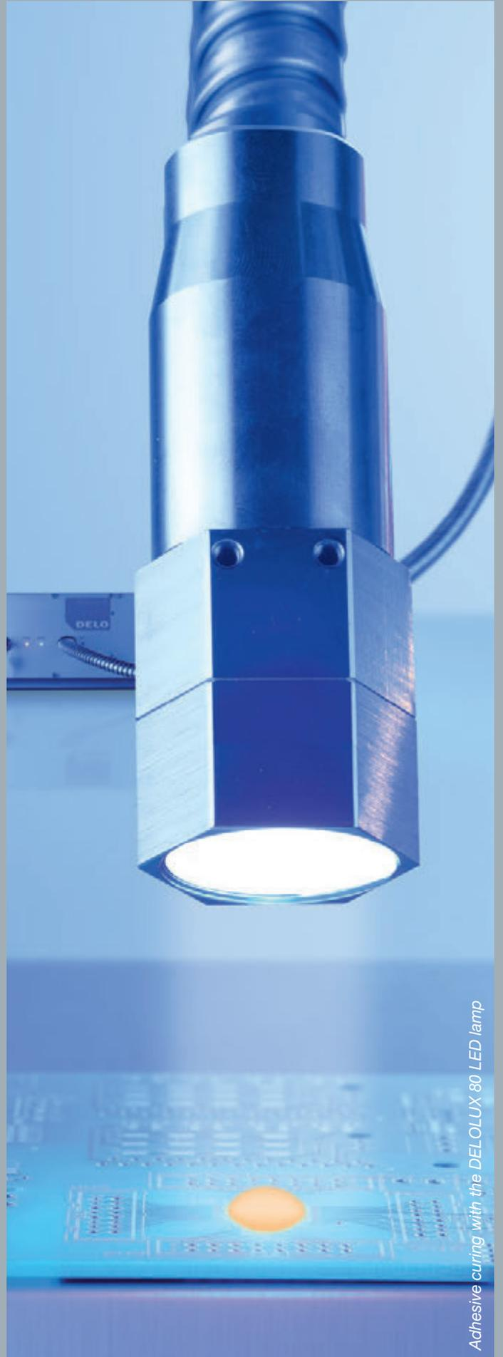
Adhesive curing with the DELOLUX 80 LED lamp
