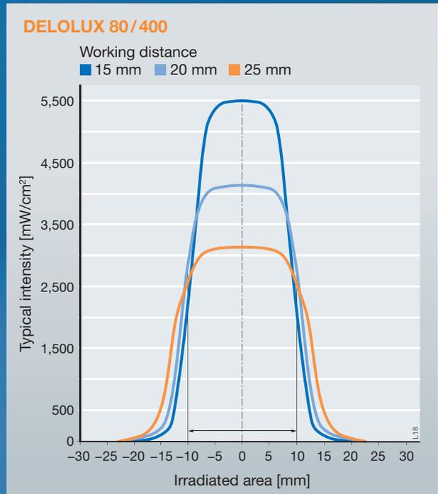
Light intensity distribution in dependence of the distance between lamp head and bonding area
