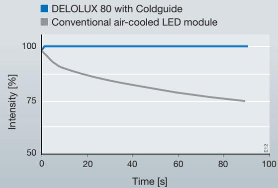
Conventional air-cooled LED module: Constant temperature, and therefore constant intensity is reached only after several minutes.
