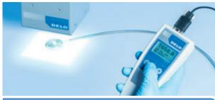
Regular intensity measurements on the component with DELOLUXcontrol for quality assurance ensure long-term process reliability.
