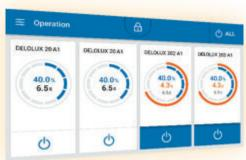
**Process control:** Irradiation parameters of up to 4 lamp heads are displayed simultaneously in the main menu and controlled via touch screen. Several user languages make the device ideally suited for international use.
