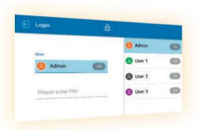
**User management:** Modification of parameters during operation is password-protected based on assigned rights. You can create individual user profiles with distinct access rights to guarantee consistent processes.
